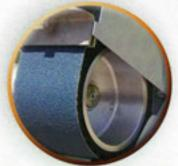
Imrpoved concave wheel with rubber carvings to allow air passage and grain opening
