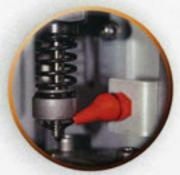
Automatic cutting oil dispenser For a sliding stroke
